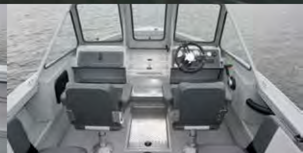
DUAL CONSOLE AND IN-FLOOR ROD STORAGE
