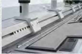
INTEGRATED GUNNEL TRACK SYSTEM (IGTS)
